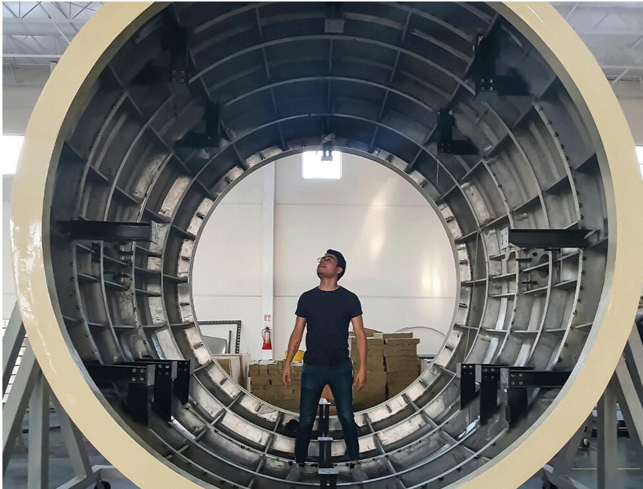
Each pod's aluminum structure, with a double curvature, showcased the firm's mastery in the hydro-forming process, utilizing a custom-made machine to shape metal with high-pressure liquid.
