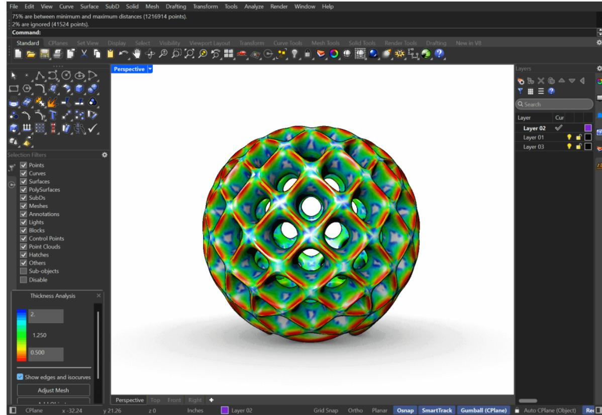
The parametric framework enabled rapid generation of multiple size variants while preserving proportional relationships and visual lightness. As the form scaled up, wall thicknesses were recalibrated to minimize weight without compromising structural integrity. The model served not only as a formal generator but as a rationalization tool, ensuring that geometry remained compatible with the constraints of powder-bed concrete printing.
