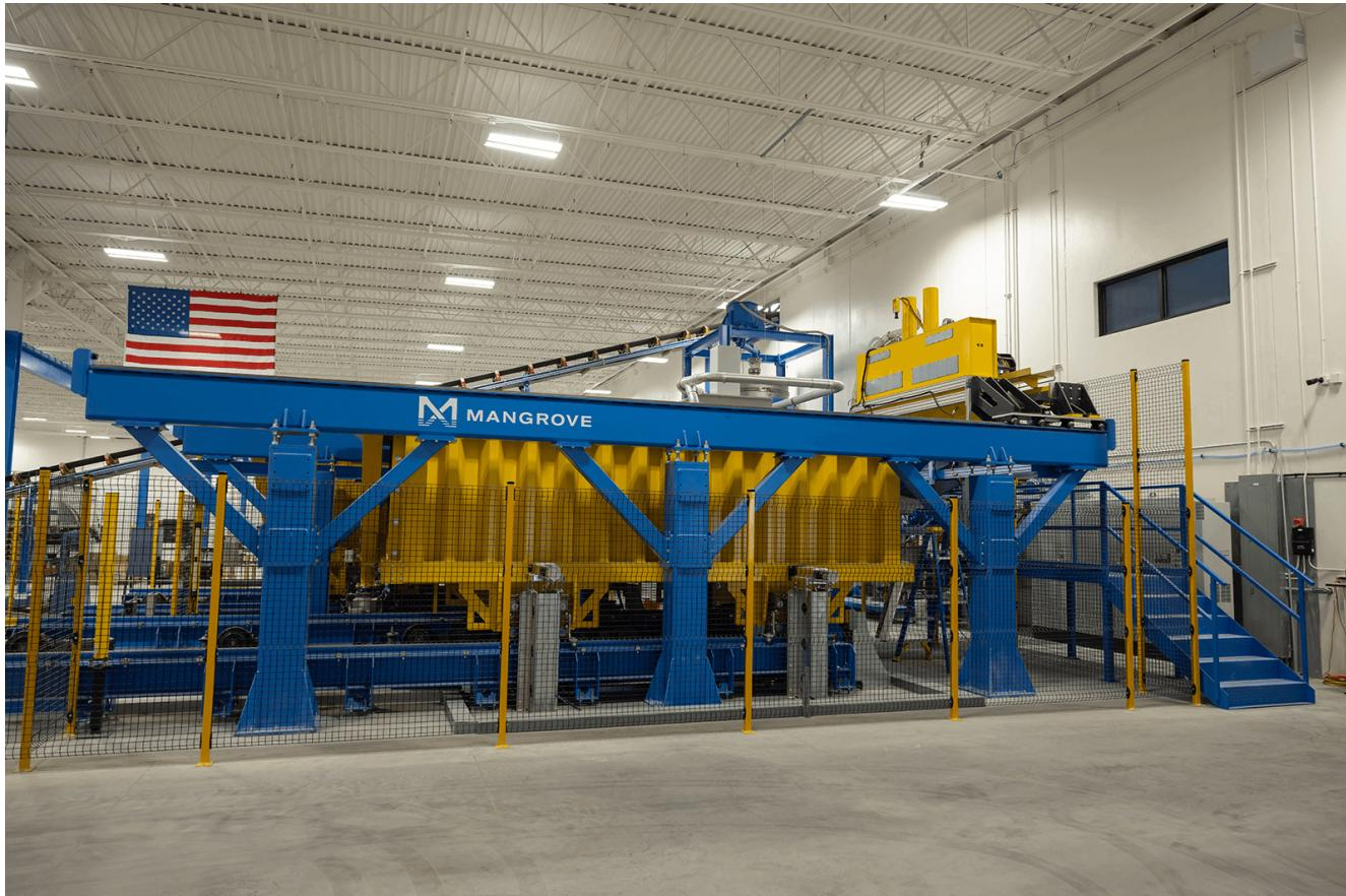
*The Balloon was fabricated using Mangrove's aggregate powder-bed concrete printing system, known as Selective Paste Intrusion (SPI).*
