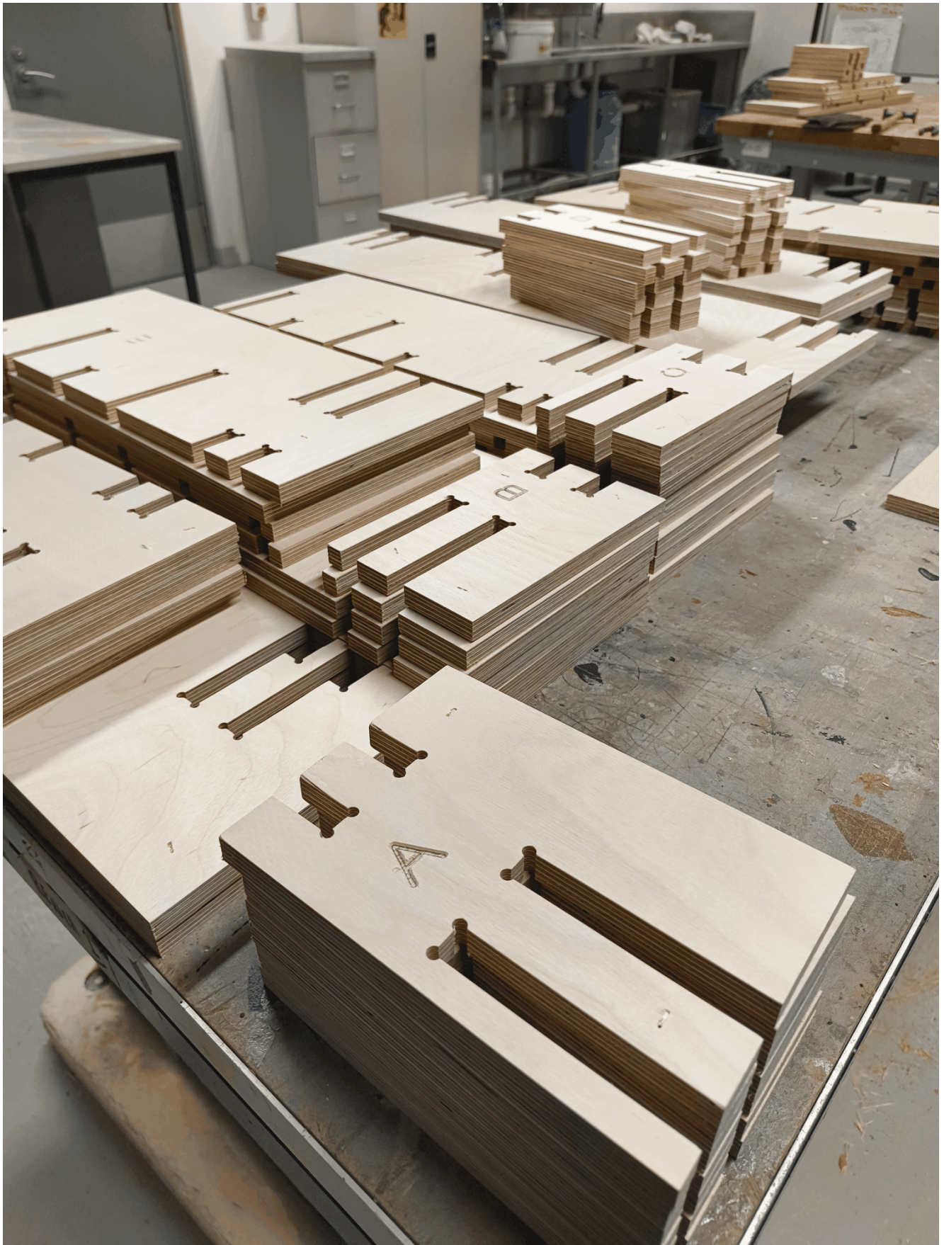
CNC-milled plywood components stacked and labelled after cutting, each slotted piece prepared to fit into the parametric interlocking system that coordinates the structure's changing geometry.
