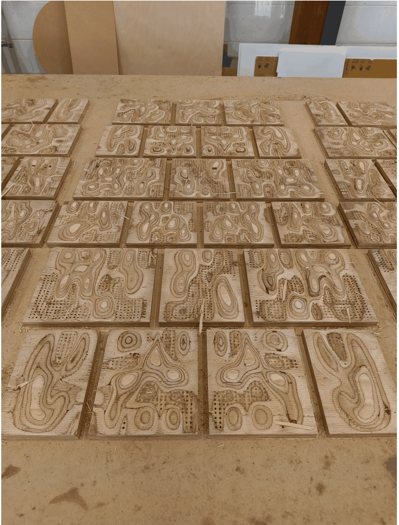
The full set of carved plywood tiles laid out together, displaying the geometric variation generated in Grasshopper and the perforations intended to contribute to sound absorption.
