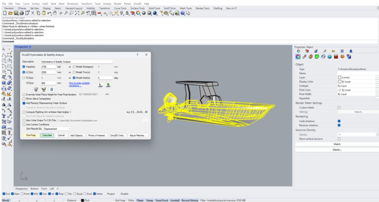
*Petestep relied on Rhino and Orca3D Marine CFD to refine the hull geometry and validate the efficiency and comfort improvements before fabrication.*
