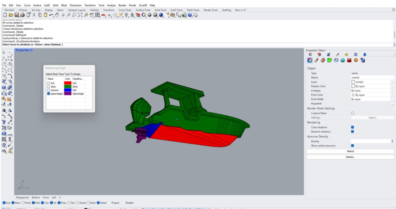
*Pestestep relied on Rhino and Orca3D Marine CFD to refine the hull geometry and validate the efficiency and comfort improvements before fabrication.*
