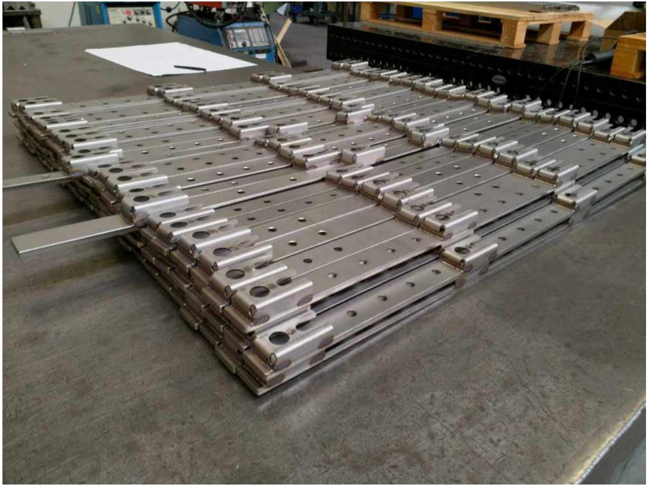
Another significant hurdle was generating accurate 2D production drawings from the 3D model. The 8mm thick laser-cut steel parts required precise bending, which was complicated by the lack of a dedicated sheet metal feature in Rhino. To overcome this, a custom algorithm was developed to account for bend factors, ensuring the parts could be manufactured correctly. Additional extensions were added to facilitate the bending process, which were manually removed before final finishing.
