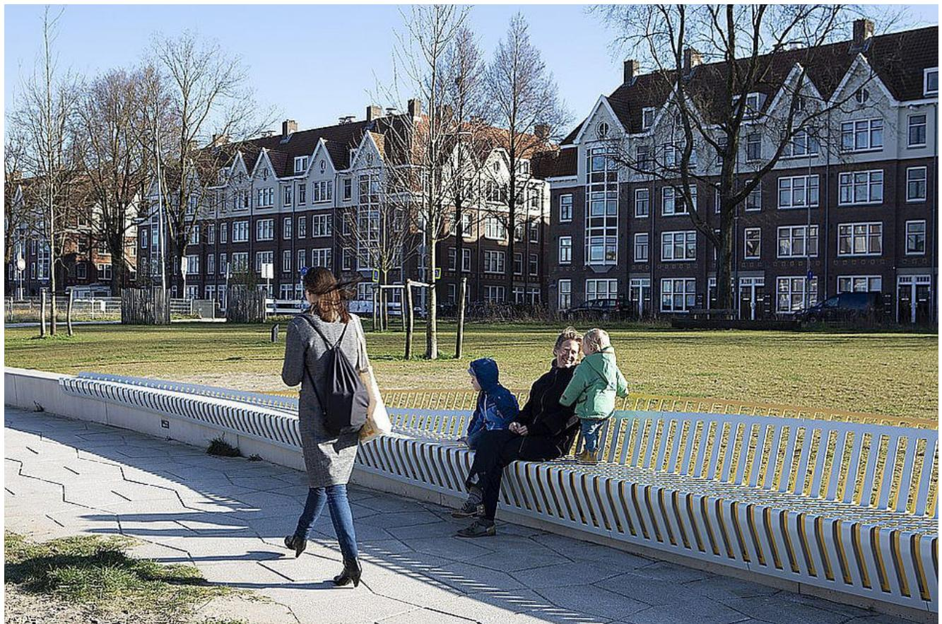
The bench's design is both intricate and dynamic. The backside modules start behind the front parts, align at seating level, and then disappear again, creating a visually engaging pattern when viewed from different angles.
