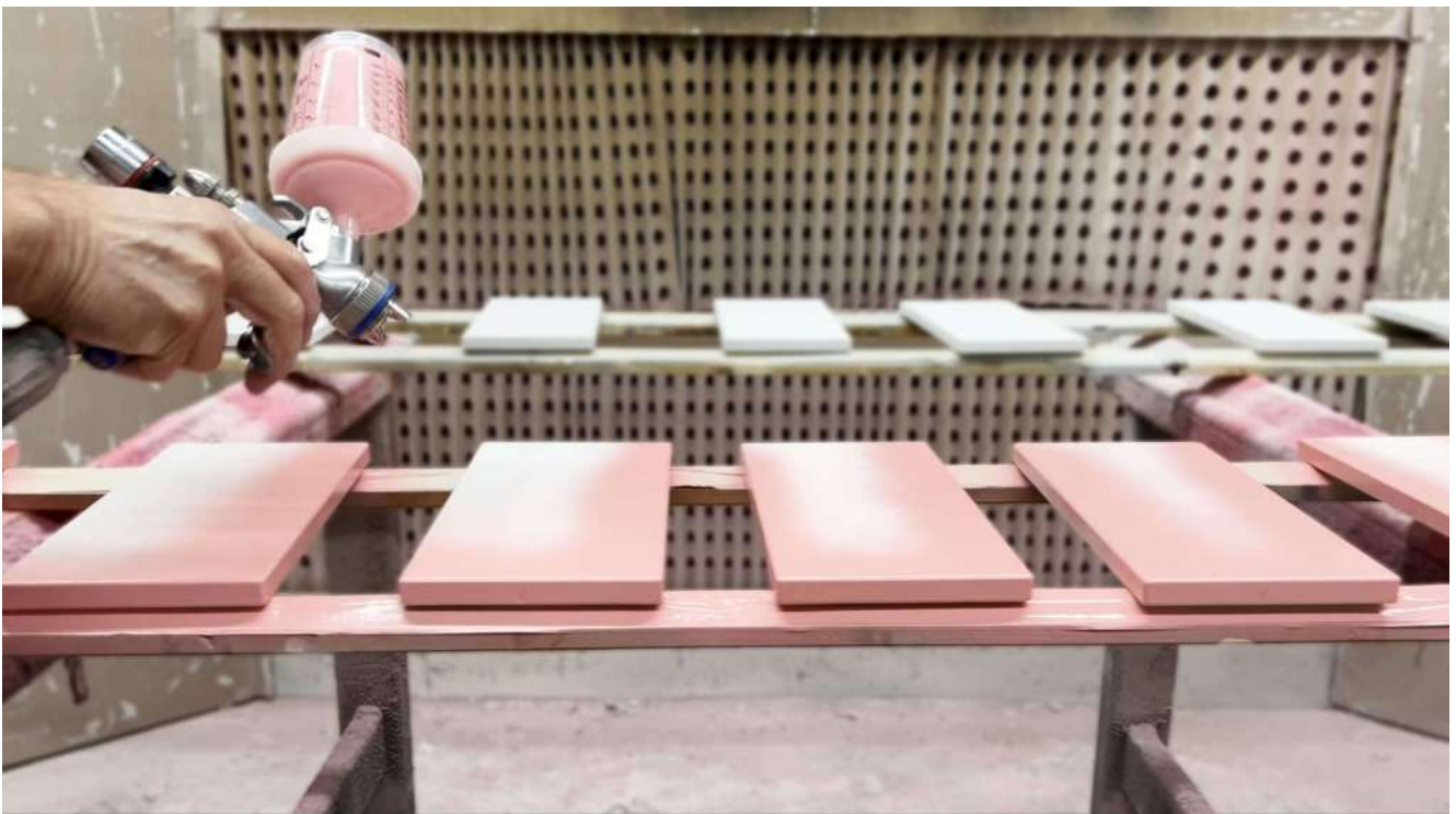
Shingles magnetic inserts and and high-quality shingle spray painting.
