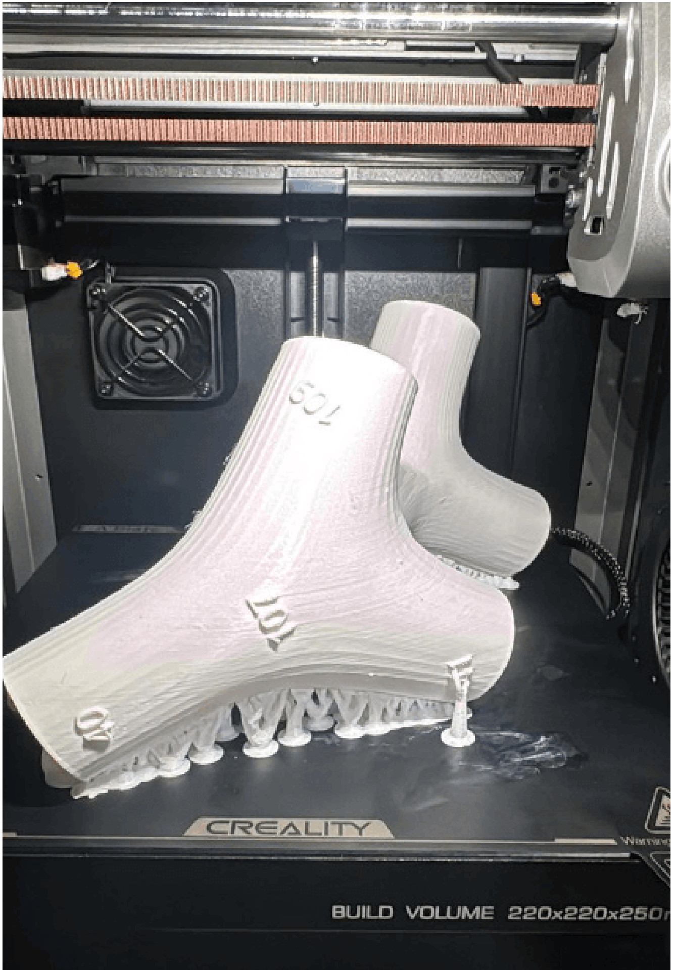
3D printing process of a custom PETG connection node
