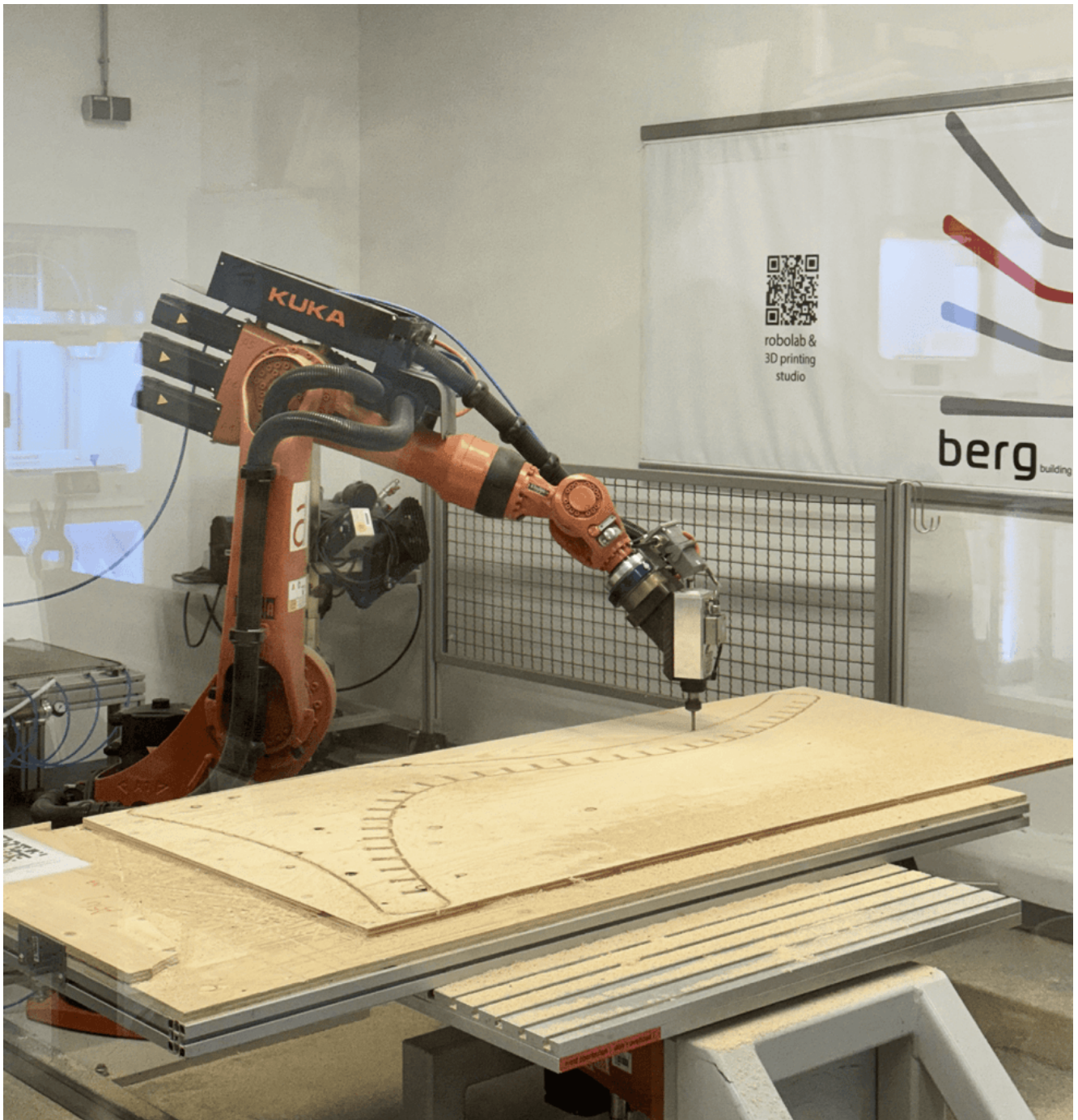
Milling and cutting with KUKA KR 16-2 robot
